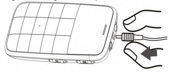
After charging finished: unplug the charger from the power socket, unplug its other end from the phone.
