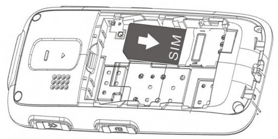
2. Remove the SIM card: hook the gap corner of the SIM card with one finger and make a lift with another finger.
