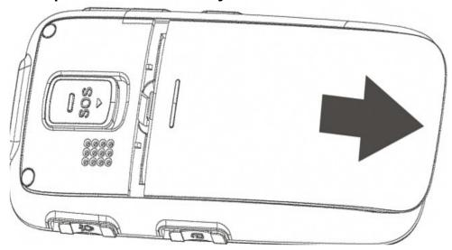
2. Put the battery in the battery slot 3 metal contact points towards back and be in line with the metal bolts at the bottom line of the cell phone, ensuring the battery's 3 metal contact points are in close alignment with the 3 metal bolts of the cell phone.
