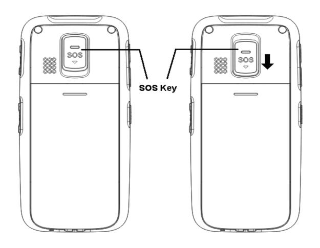
Warning: Please keep the SOS sliding switch at its initial position under Non-SOS state, if the SOS switch is already in the SOS state before turning on the cell phone, the cell phone will, at the turning-on time, ask you to confirm the SOS state of the SOS switch (if the SOS switch is not reset when the cell phone is under power-on state, you have to reset it and start-up the SOS function in case of an emergency).
