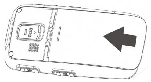
Note: Be sure to turn off the cell phone and disconnect the connection with the charger before removing the battery, and please only use batteries designed for this type of cell phone.
